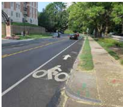
Right: Bicycle lanes can help to narrow roadway width, slowing down automobiles while providing bicycles with a space to travel.
