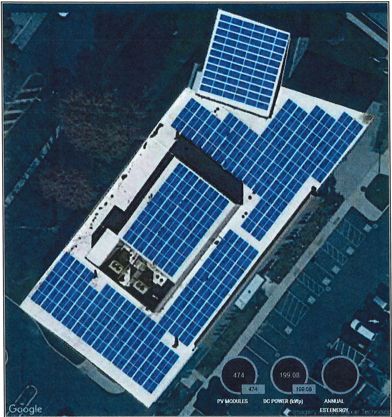
Figure 3 Springfield TWP Admin / Police Building Array Layout
