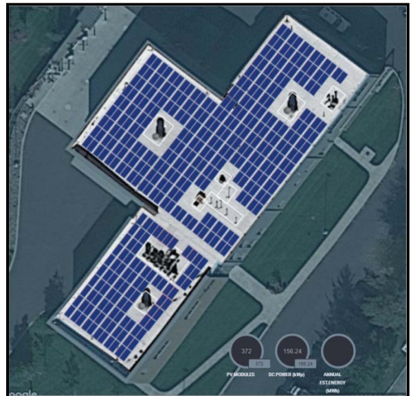
Site 2.1 - PW Main Building – 156.24 kW DC
