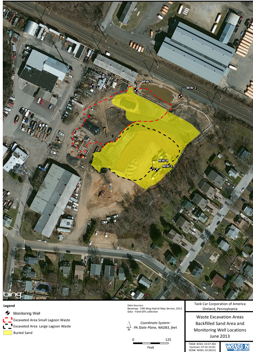
Waste Excavation Areas, Backfilled Sand Area and Monitoring Well Locations by Weston Solutions 06/2013
